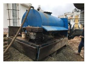
Figure 3: Desludging vehicle; a tank equipped with movable centrifugal pump on a truck.
