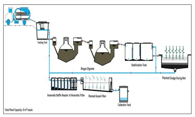
Figure 2: Overview of FS treatment technology of Lubhu FSTP (source: ENPHO).
