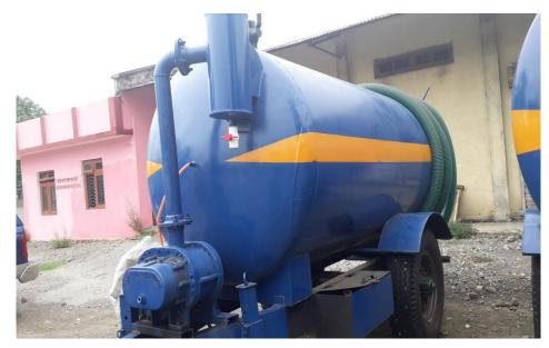
Figure 12: A newly purchased desludging vehicle by the Bheemdatt Municipality.
