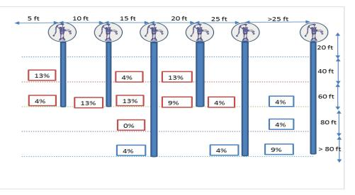
Figure 10: Depth of hand pumps and lateral spacing of it with containment type lined tank with impermeable wall and open bottom.
