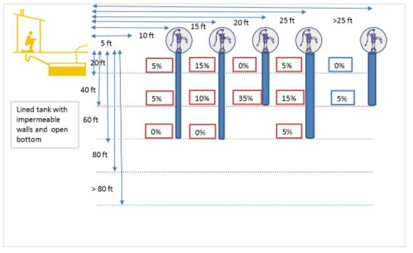
Figure 12: Depth of hand pumps and lateral spacing of it with containment type lined tank with impermeable wall and open bottom.
