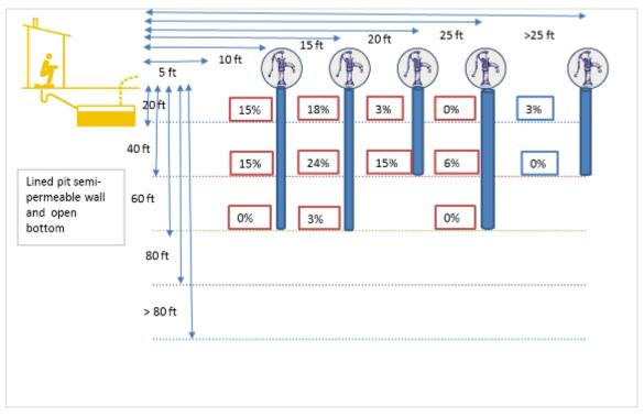
Figure 13: Depth of hand pumps and lateral spacing of it with containment type lined the pit with semi-permeable wall and open bottom.
