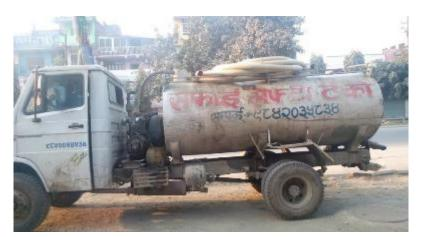
Figure 6: Locally assembled mechanized emptying vehicle
