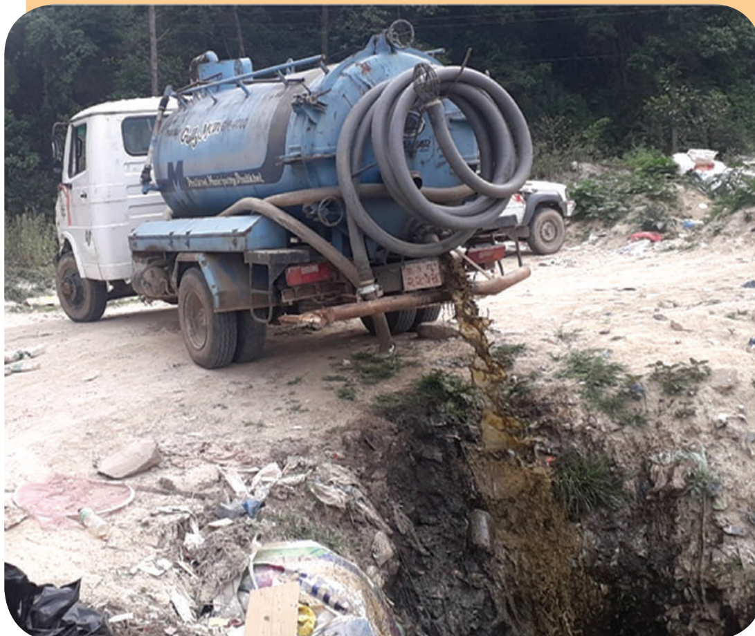
Figure 13 Direct disposal of FS in landfill site
