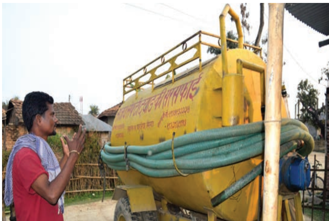
Figure 14 Locally manufactured desludging vehicle operated by private entrepreneur
