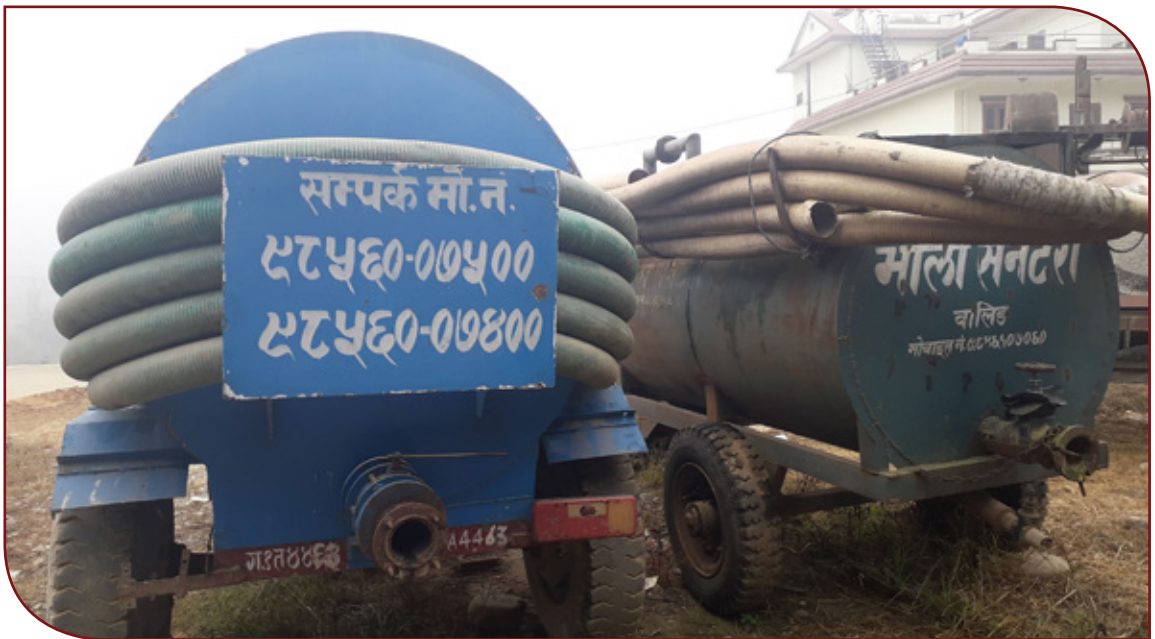
Figure 10: Desludging tanker operated by private service provider
