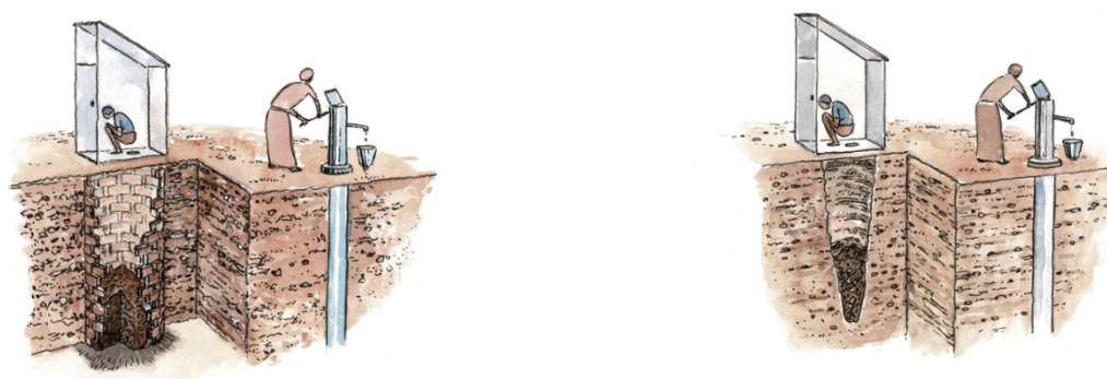
Figure 8: Lined pit with semi-permeable walls and open bottom, no outlet or overflow (left) and Unlined pit, no outlet or overflow (right).
