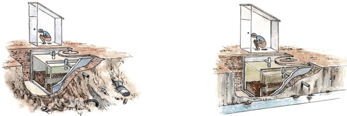
Figure 5: Septic tank connected to open drain or storm water (left) and Septic tank connected to open ground (right).
