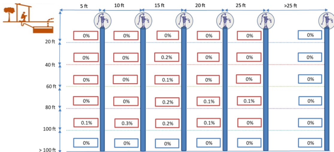
Figure 19: Groundwater contamination risk from lined pits with semi-permeable walls and open bottom.
