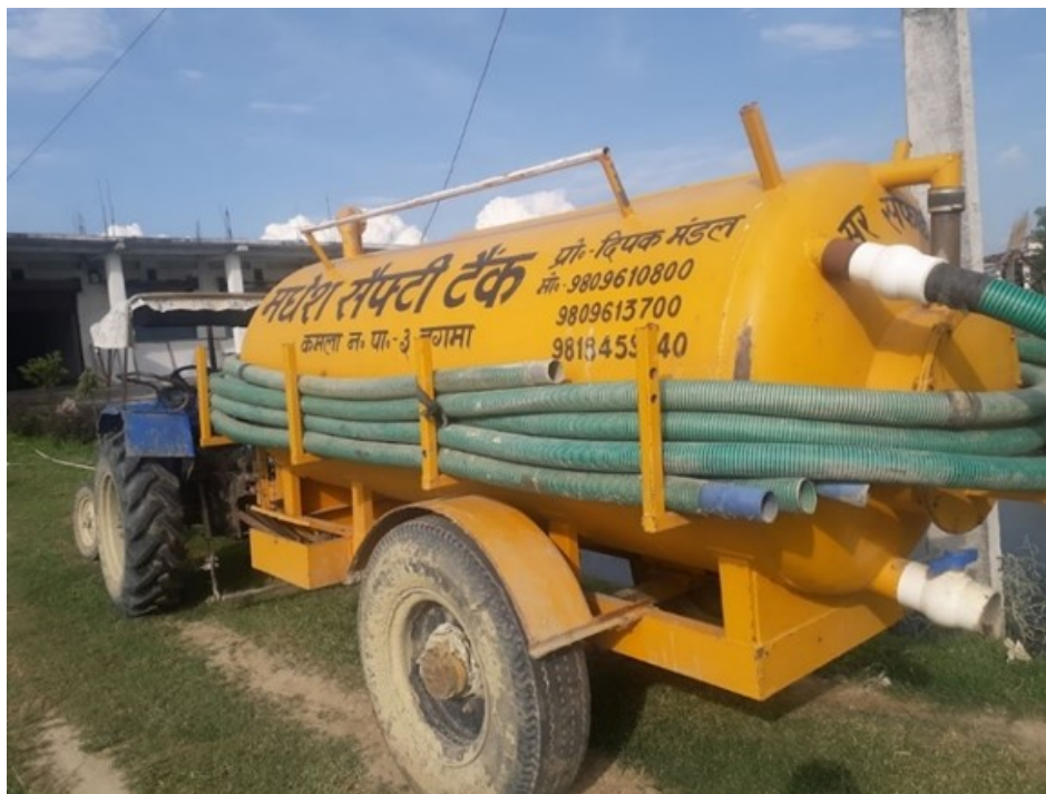
Figure 7: Mechanical emptying of the containment in Dakneshwori Municipality.
