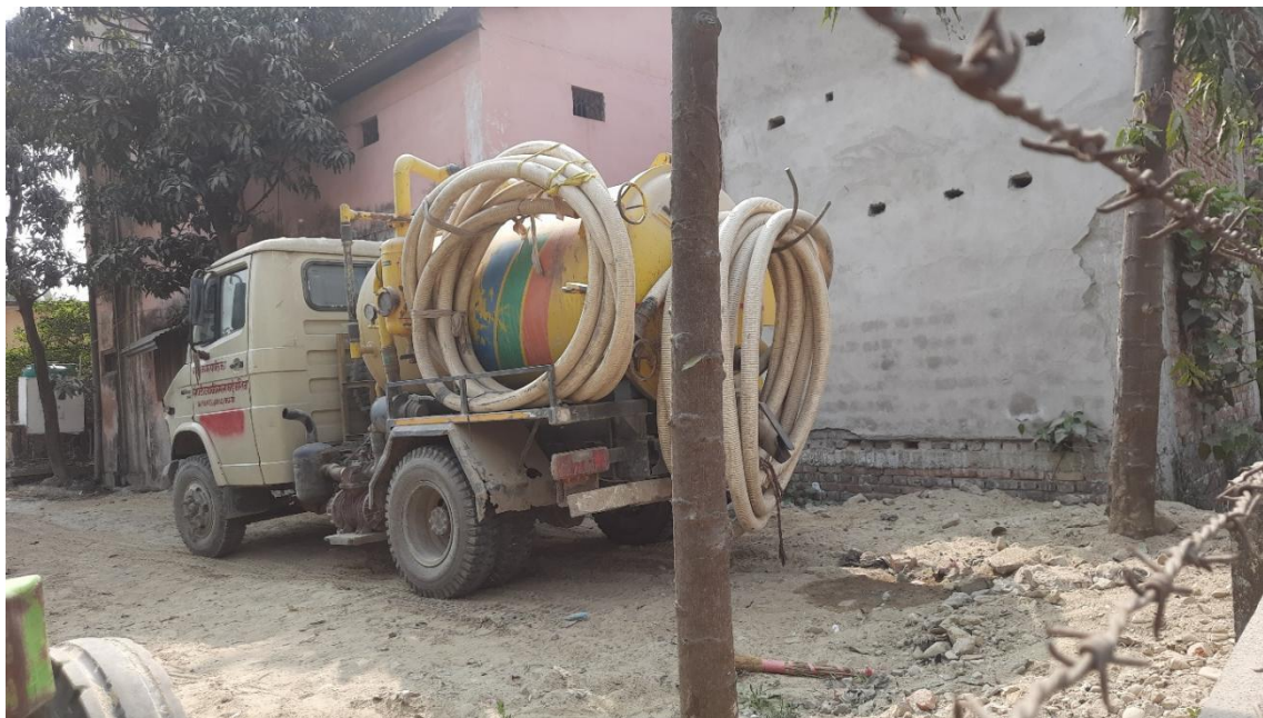
Figure 12: Mechanical emptying vehicle operated by Gaur Municipality.
