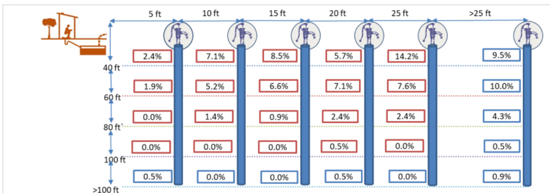
Figure 17: Depth of hand pumps and lateral spacing of it with containment types: lined pit with semi-permeable walls and open bottom.
