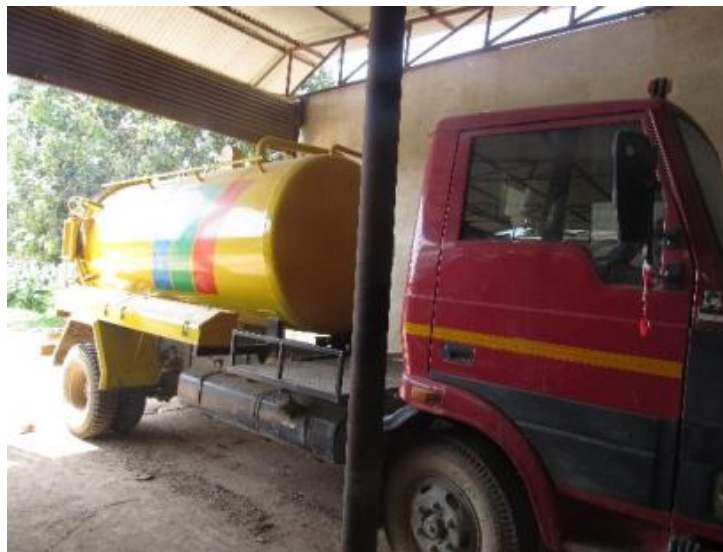
Figure 13: Municipal desludging vehicle for emptying of the containment in Gulariya Municipality.
