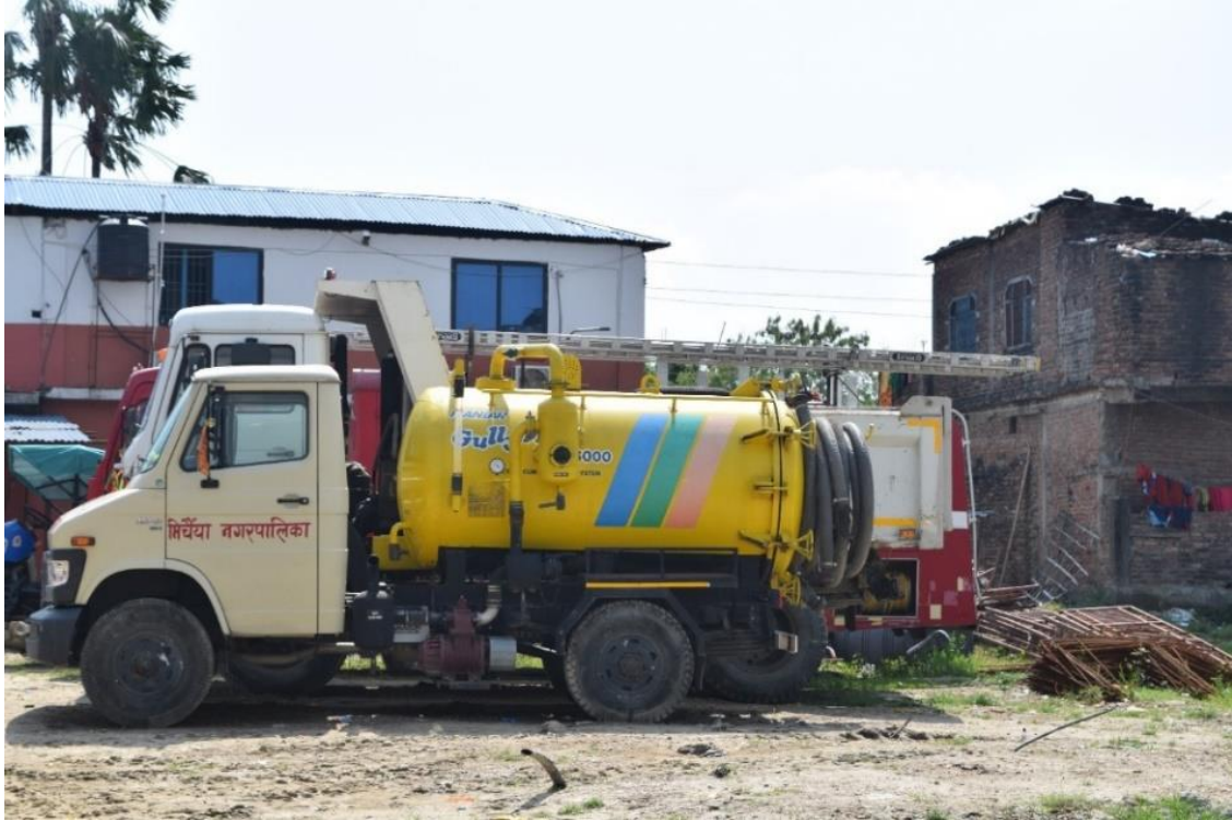
Figure 13: Desludging vehicle of the Mirchaiya Municipality.
