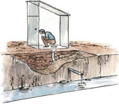
Figure 4: Toilet discharges directly to open drain.
