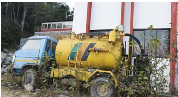
Desludging vehicle of Bhimeshwor Municipality
