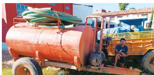
Municipal desludging vehicle
