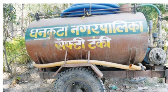
Municipal desludging vehicle
